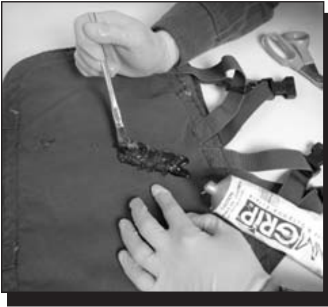
Figure 7—Spread Seam Grip over the entire hole.
