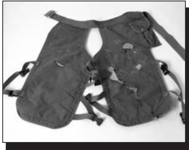
Figure 3—Retire chaps when they have numerous holes and cuts.
